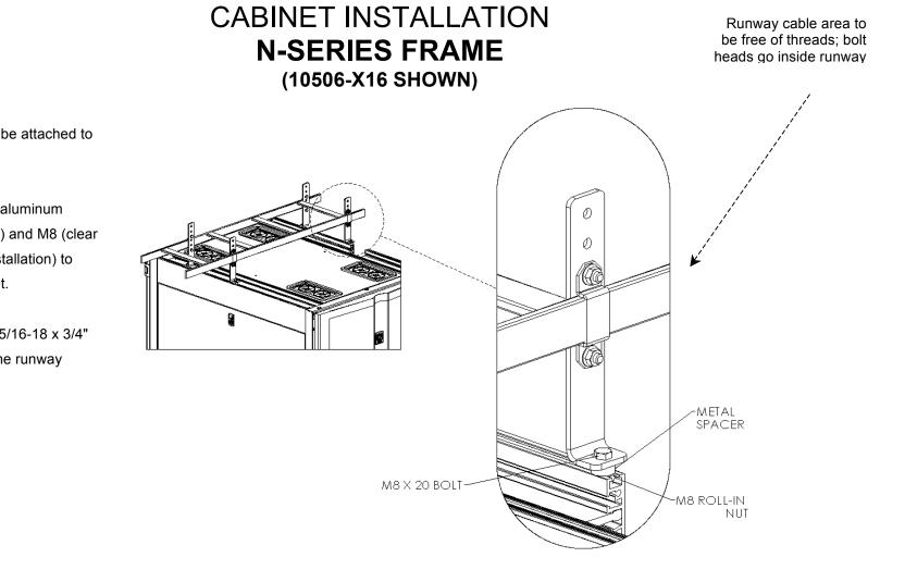
Elevation Brackets should be attached to the outer slides.
