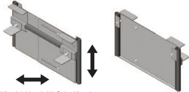
Adjusts in height and width. Back and front shown.
