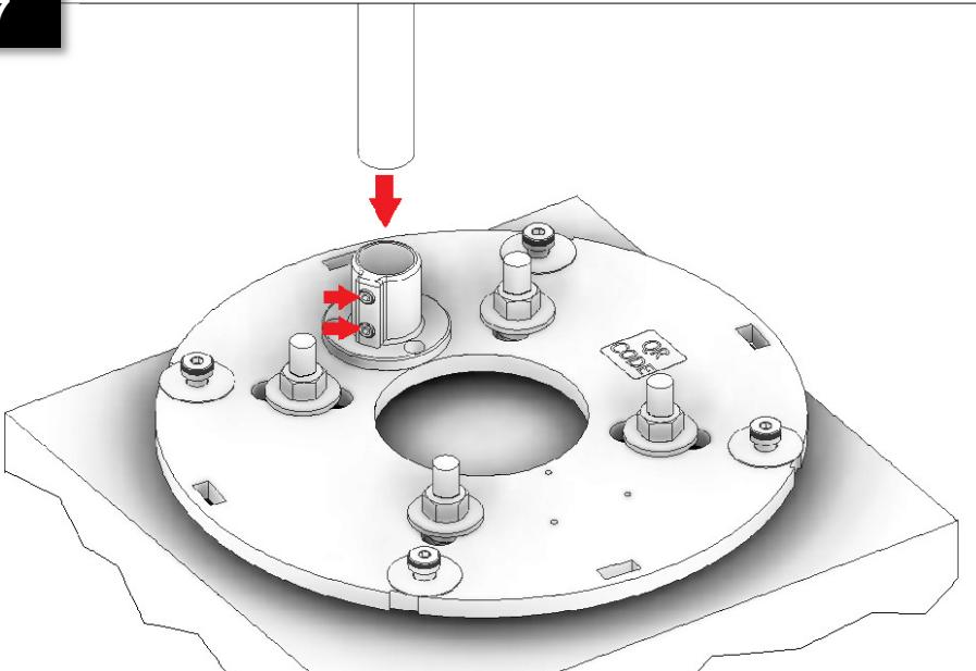
Insert the steel pole into the Aluminum Pole Flange to the Anchor Base. Tighten the set screws to secure the steel pole in position.
