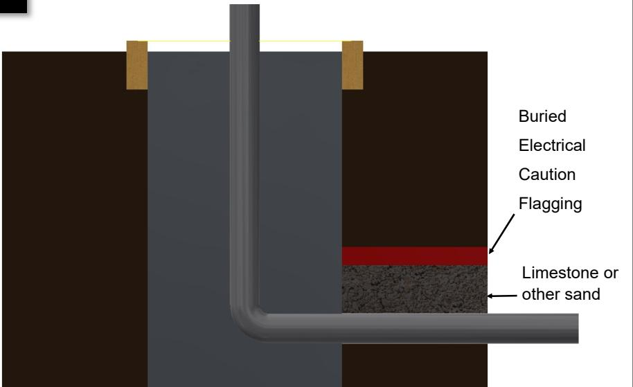
Follow local code requirements for buried conduit. Fill around the conduit with gravel if necessary. Mix and pour the concrete around the conduit. 3000 to 3500 psi concrete is recommended.
