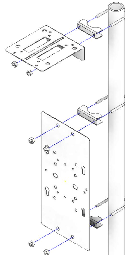
Determine which mounting bracket(s) to install to the pole. Most Aruba access points will require the right angle bracket and most Cisco access points will require the vertical bracket (Note: depending on what equipment is being installed, some installations may require both) Remove the nuts and clamp from the U-Bolt and place the U-Bolt around the pipe. Install the clamp, mounting plate and nuts as shown in diagram. Securely tighten the nuts.
