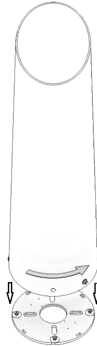
Verify the bollard tube is seated properly on the anchor base (the anchor base should not be visible when viewed from the side). Looking from the top, rotate the bollard tube counter clockwise until it stops (approximately 10°). Insert the key and rotate counterclockwise to engage lock. Verify the lock is fully engaged by rotating the tube back clockwise, it will have about 1° to 2° play. If the lock did not fully engage, re-align and verify the tube was properly seated on the anchor base.
