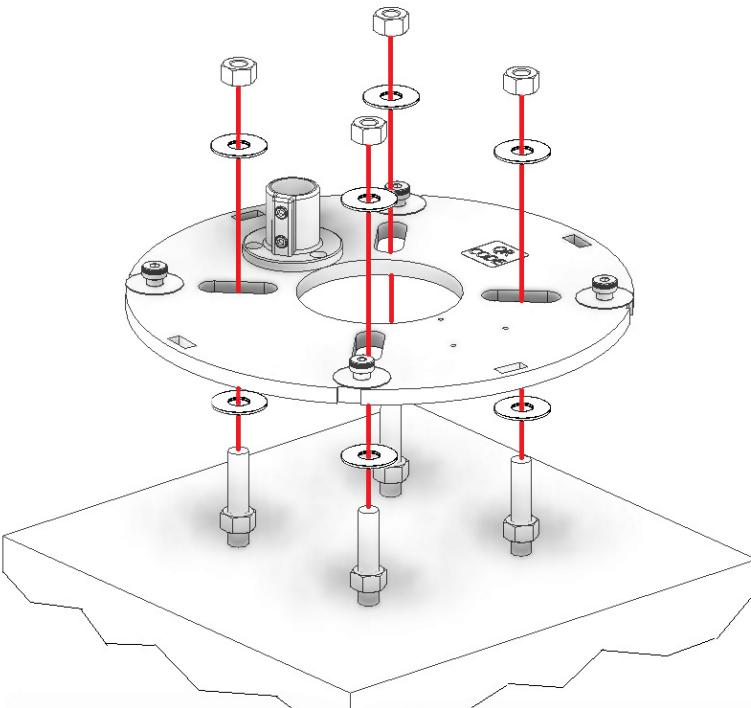
After the concrete has set, remove the bolt positioner board. Leave the lower nuts and washers in place for anchor base installation.
