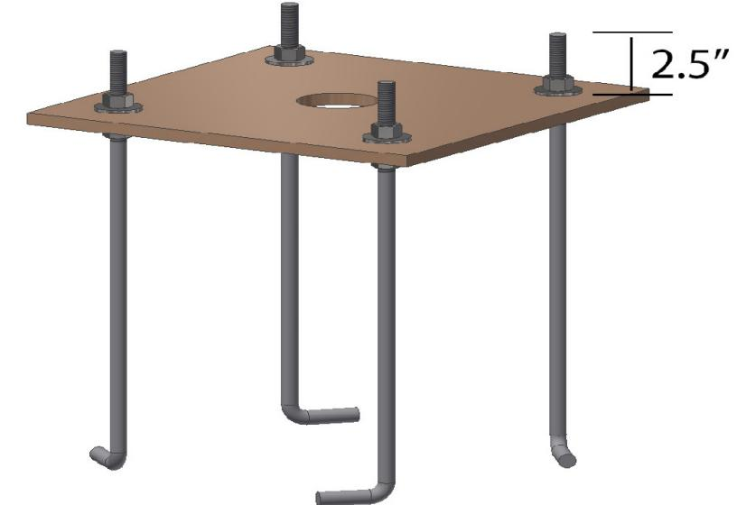
Create a bolt positioner board to hold anchor bolts in place while the concrete sets and drill a center hole large enough for conduit. Fasten 5/8" x 18" anchor bolts in a 6" x 6" square to the board using 5/8" nuts and washers above and below, leaving 2.5" or greater above the board. Oberon's 39-303X-FOOTING KIT includes bolts, and hardware for anchor bolt positioning. The bolts must be tight to prevent them from migrating while installing.
