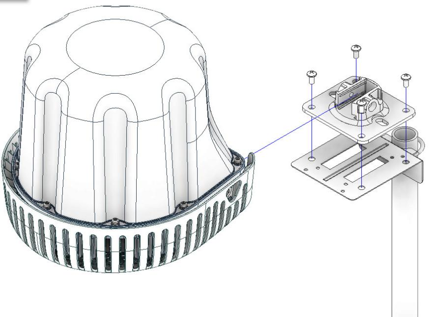
Most Aruba access points are to be mounted horizontally. To mount Aruba access points in the 3036 bollard, use the Aruba "H2" mounting bracket purchased from Aruba. The right angle mounting bracket has hole locations available to mount the H2 bracket. First attach the H2 bracket to the right angle bracket then attach the Aruba access point to the Aruba mounting plate following manufacturer's directions.
