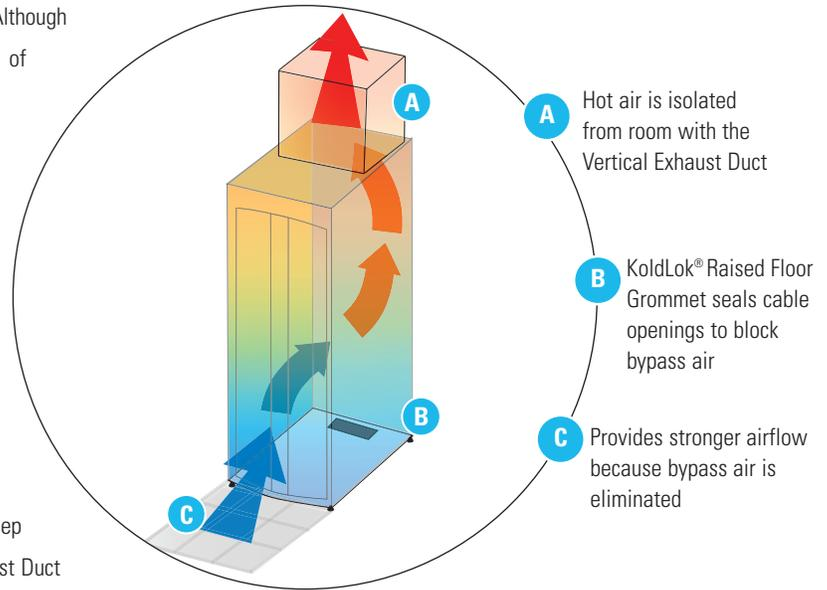
the office and data center operating at comfortable temperatures. In addition, the fact that CPI's solutions keep hot exhaust and cool supply air separated, makes AC unit failure much less of an issue, especially since we only use it during the warmer months," explained Julian.
