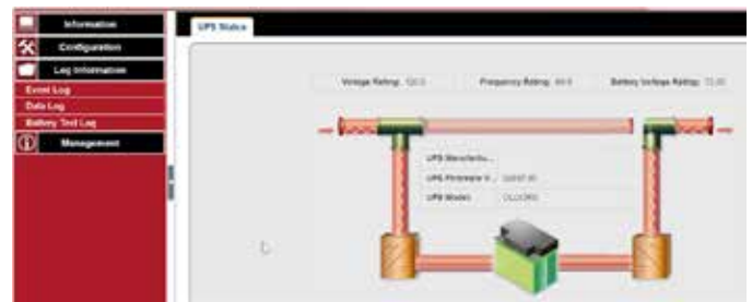
FIGURE 2: Intelligent UPSs report voltage, frequency, waveform, battery capacity, and other critical information.
