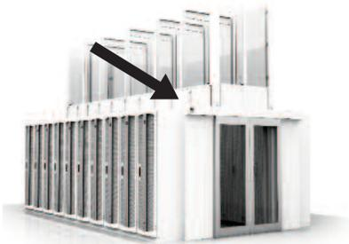
Adjustable Height Filler Panels (20 shown) attached to the Frame-Supported Exhaust Duct. Panels are used above each cabinet to fill the gap between the cabinet and the 52U high frame/duct.
