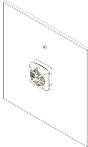
**Figure 5** – Proper positioning of AP within the 1068 enclosure. Note that the access point should be located within the AP mount so that the LED is located facing away from the lock
