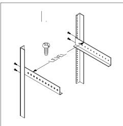
MOUNT REAR BRACKETS TO REAR MOUNTING RAILS AS SHOWN ABOVE, WITH TWO EACH 12-24 PAN-HEAD MOUNTING SCREWS.
