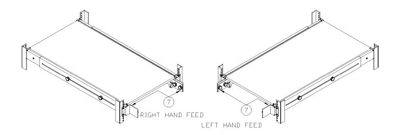
(7.) INSTALL CABLE MANAGER WITH DESIRED CABLE FEED ORIENTATION AS SHOWN.
