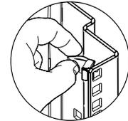
Align, squeeze, insert and release.
